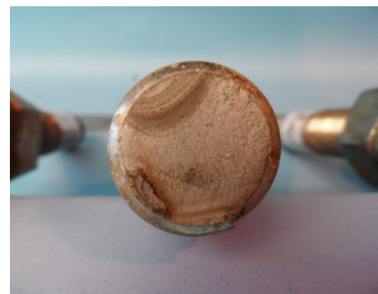
Example of progressive fatigue type failure
