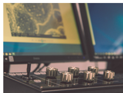
Imaging can be carried out using high vac and low vac using a range of detectors
